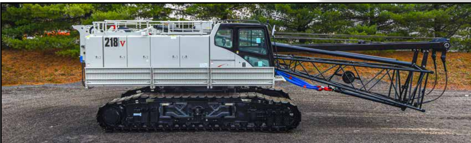
Counterweights lower completely to the ground
