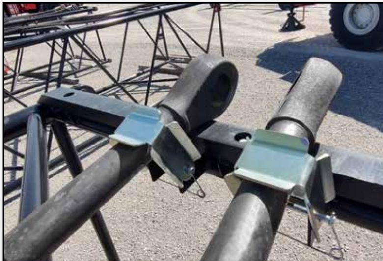
New pendant storage on every section of boom
