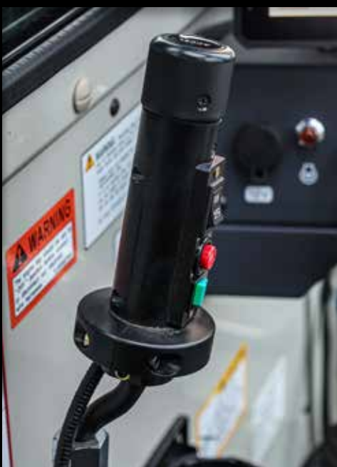
Variable hand throttle for infinite main pump control.
