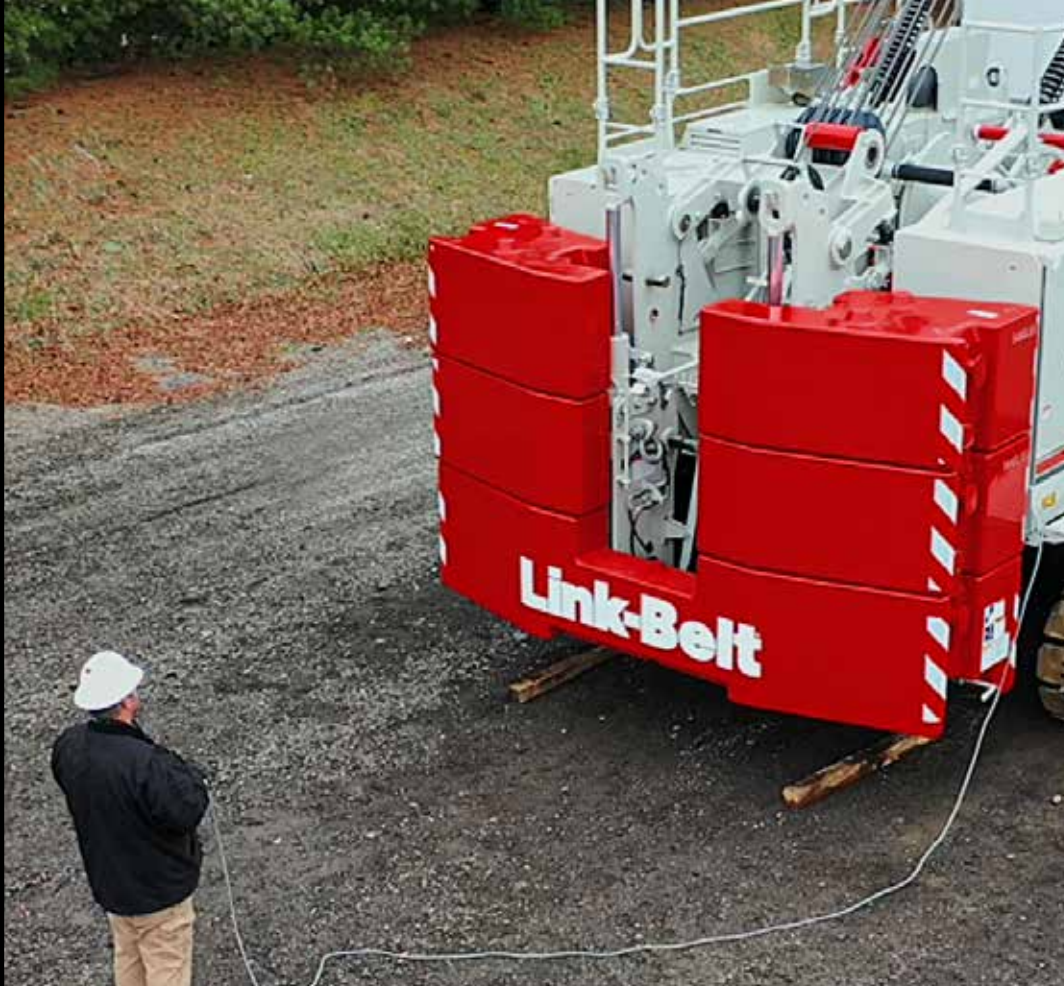
Counterweights lower completely to the ground
