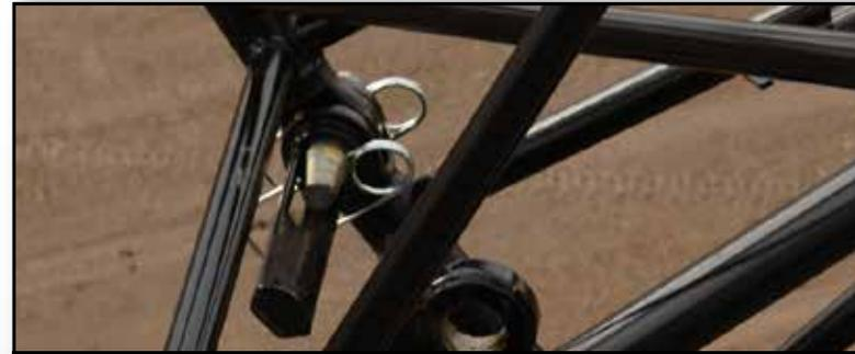
Double tapered connecting pins for installation/removal from outside of boom. Boom connecting pins store in pin catchers for transport.
