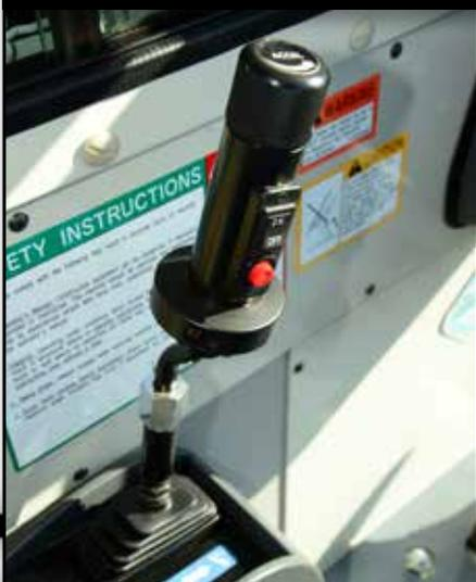
**Pilot-operated armchair controls** with adjustable sliding console
