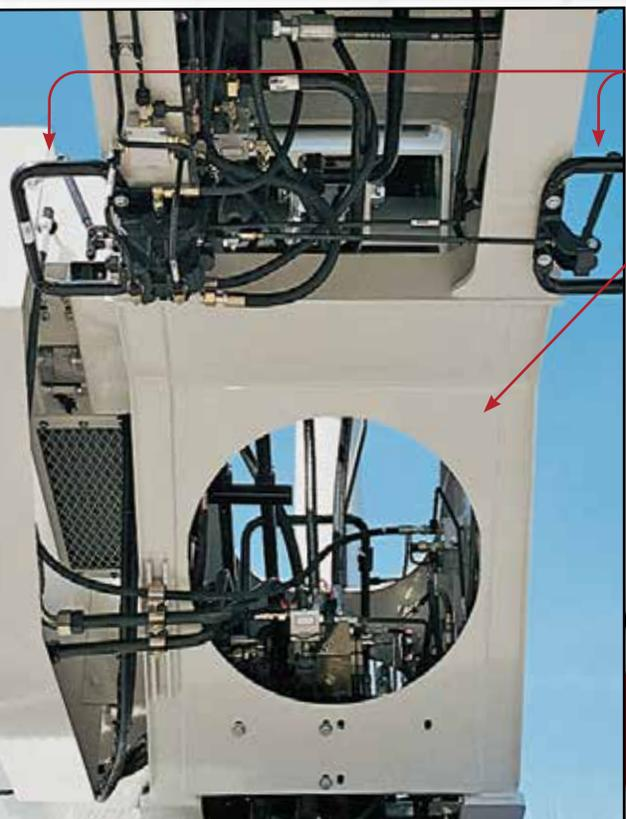
• **Counterweight transfer removal controls** located on each side of the upper structure.
