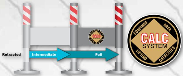
**The Confined Area Lifting Capacities (CALC)** system provides three outrigger positions:
