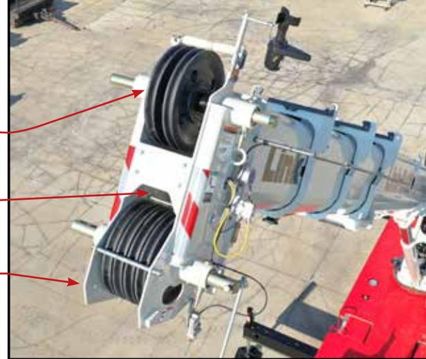
**Hammerhead boom** nose allows the operator to work at high boom angles without fouling wire rope.
