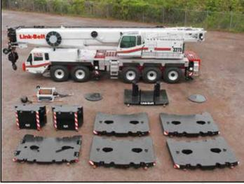
^ Auxiliary winch can be removed and installed without an assist crane using only the bottom tray of the counter weight stack. A newly designed counterweight removal system allows all counterweight configurations to be raised and lowered by hydraulic cylinders from the comfort of the operator's cab.
