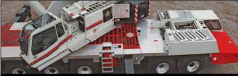
Access to the engine compartments and the operator's cab is superb with strategically-located ladders and steps.
