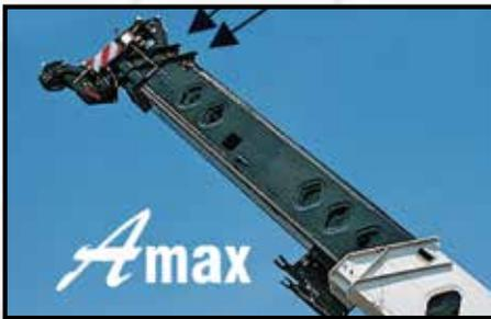
Exclusive **Amax mode** (mode “A”) offers substantially increased capacities. **Standard mode** (mode “B”) self-proportions all four sections equally.
