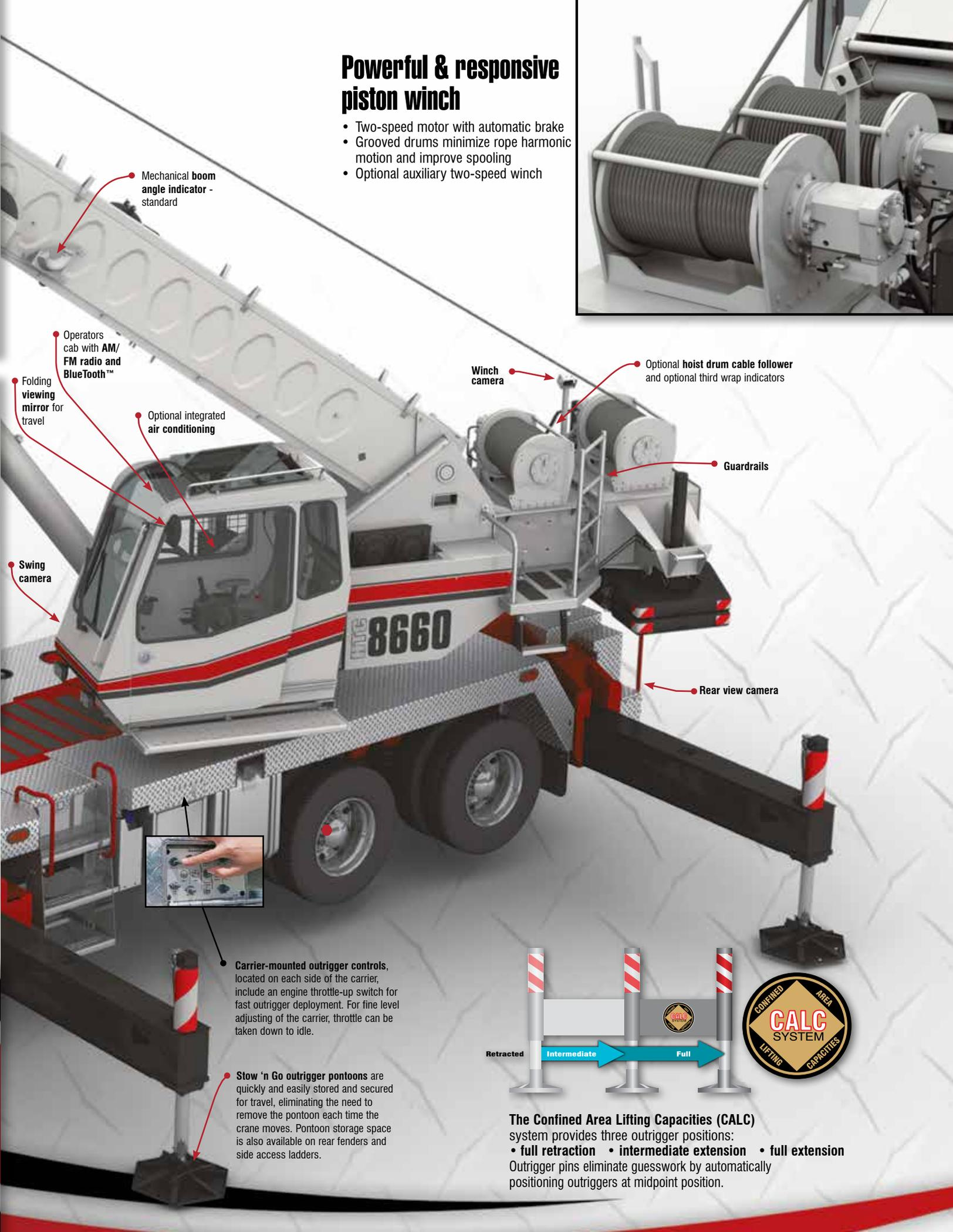
Mechanical boom angle indicator - standard
