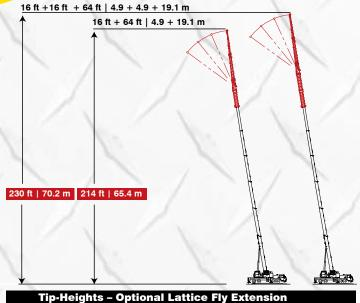
The optional 64 ft | 19.51 m two-piece offsettable bi-fold fly can be extended by adding up to two optional **16 ft | 4.9 m lattice inserts** with  $2^{\circ}$ ,  $15^{\circ}$ ,  $30^{\circ}$ , and  $45^{\circ}$  manual offsets.
