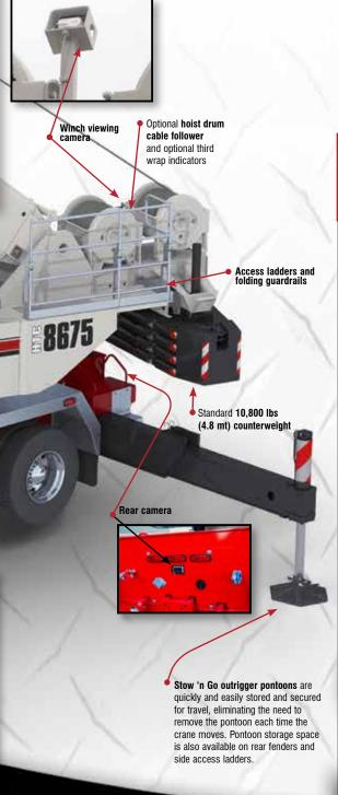
The Confined Area Lifting Capacities (CALC) system provides three outrigger positions:
