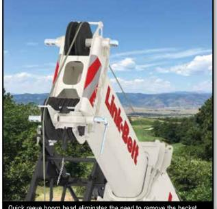
Quick reeve boom head eliminates the need to remove the becket when it becomes necessary to change the reeving.
