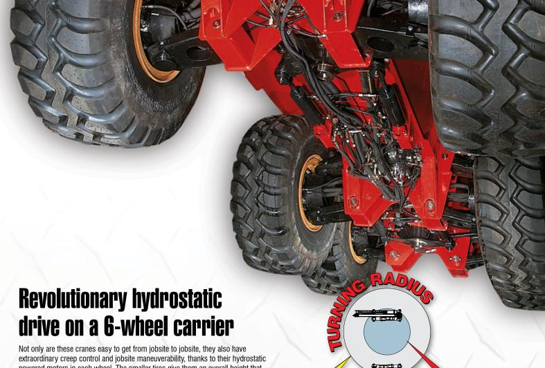
Not only are these cranes easy to get from jobsite to jobsite, they also have extraordinary creep control and jobsite maneuverability, thanks to their hydrostatic powered motors in each wheel. The smaller tires give them an overall height that is ideal for hauling, along with their individual six-wheel hydrostatic drive. There is no crane in the world, any size, that can come close to the job site maneuverability and performance of Link-Belt's large RTC Series II machines.
