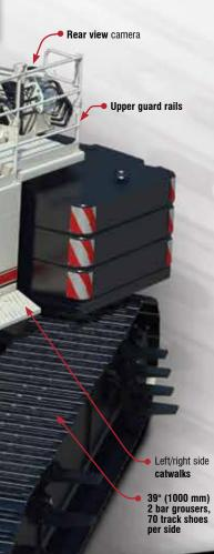
Sealed oil-filled idlers upper and lower rollers
