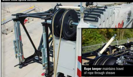
Quick reeve boom head eliminates the need to remove the becket when it becomes necessary to change the reeving
