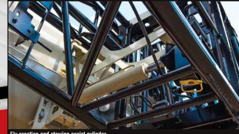
Fly erection and stowing assist cylinder
