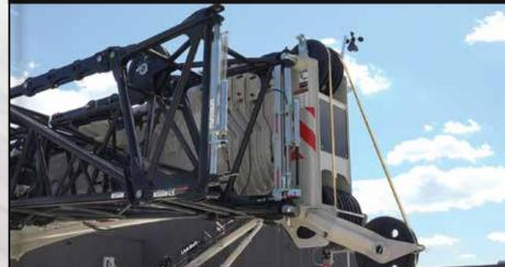
New efficient fly pinning design focuses on ease of assembly/disassembly
