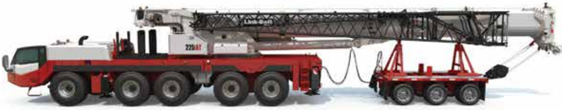
Boom dolly/trailer ready - boom connections, air & electrical, boom float & free swing
