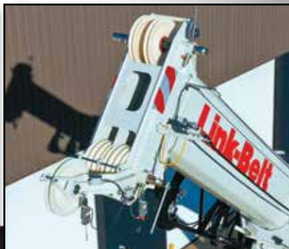
Quick reeve boom head eliminates the need to remove the bucket when it becomes necessary to change the reeving
